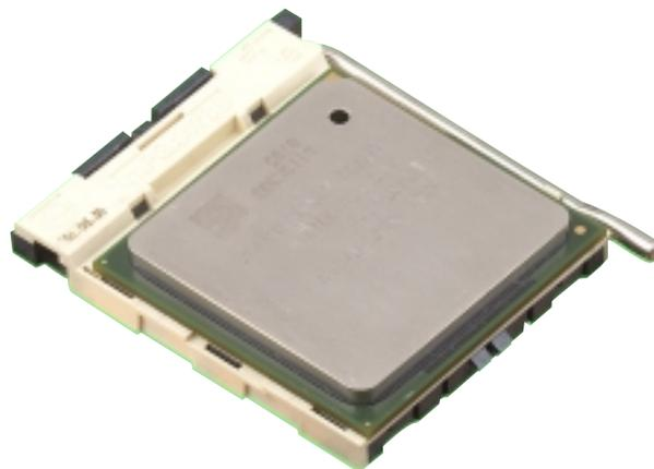
Figura 2-8 CPU Instalada
