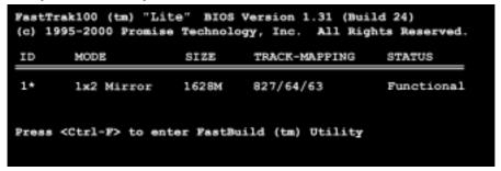
8. If duplicating an original Operating System to another new hard disk, the system will start up automatically. If creating a brand new RAID 1 array only, it will be necessary to intstall a new OS. Reboot with a rescue floppy disk to format the hard disks with the *FDISK* command and then install the OS from a CD; alternatively, with a *bootable* OS CD, install the new OS automatically.
