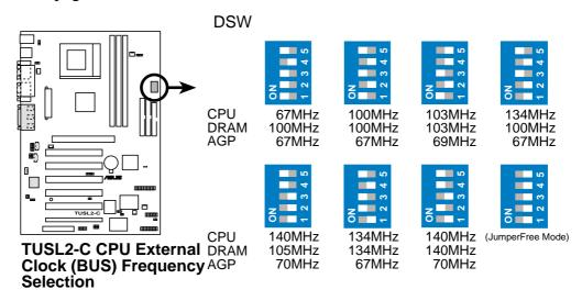
**NOTE:** If your processor does not have a locked Frequency Multiple, you must use **CPU Core:Bus Freq. Multiple** in *4.4 Advanced Menu* to set the Frequency Multiple. If the Frequency Multiple is locked, setting the Frequency Multiple in BIOS setup will have no effect.
