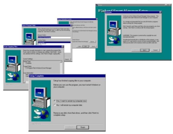
The auto-installer implements all of the drivers, base components and displays the Winbond Smart Manager program groups. **Restart**. Windows should auto-detect the smart card reader and install its system drivers.
