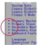
certain fields. This pointer indicates that a sub-menu can be launched from this field. A sub-menu contains additional options for a field parameter. To call up a sub-menu, simply move the highlight to the field and press <Enter>. The sub-menu will then immediately appear. Use the legend keys to enter values and move from field to field within a sub-menu just as you would within a menu. Use the <Esc> key to return to the main menu.
