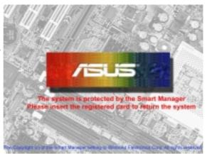
3. **Always Check** configures the *Smart Manager* to require that the user insert the smart card during start up; then, if the card is removed at any time during the operation of the PC, the *Smart Manager* protection screen will automatically pop up and the PC is secure until the card is reinserted.
