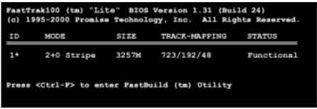
6. To finish installation of your new Operating System to the RAID 0 array, reboot with a floppy disk to format the hard disks with the *FDISK* command and then install the OS from a CD; alternatively, with a bootable OS CD, you may install the new OS automatically. As you install the OS, the system always treats the RAID 0 array of hard disks as if they are a single drive unit.
