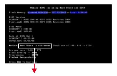
**NOTE:** When you see the message "Boot Block is different", you may still press <Y> to update the BIOS. Yet if the update fails, your system will run a greater risk of boot failure depending on whether the boot block is damaged or not.
