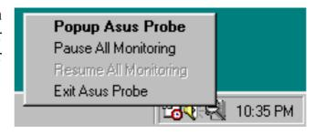
When the ASUS PC Probe senses a problem with your PC, portions of the ASUS PC Probe icon changes to red, the PC speaker beeps, and the ASUS PC Probe monitor is displayed.
