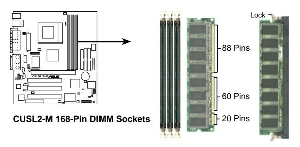
The DIMMs must be 3.3Volt unbuffered SDRAMs. To determine the DIMM type, check the notches on the DIMMs (see figure below).
