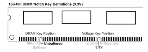
The notches on the DIMM will shift between left, center, or right to identify the type and also to prevent the wrong type from being inserted into the DIMM slot on the motherboard. You must tell your retailer the correct DIMM type before purchasing. This motherboard supports four clock signals per DIMM.
