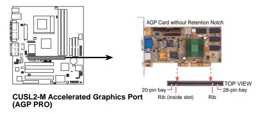
**NOTE:** Disable the integrated graphics controller (see **Onboard VGA** in *4.4.1 Chip Configuration*) when using an add-on graphics card.
