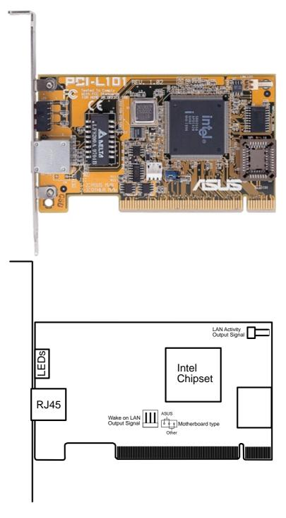
If you are using the ASUS PCI-L101 on an ASUS motherboard, leave the jumper on its defaut setting of "ASUS." If you are using another brand of motherboard, set the jumper to "Other." Connect the Wake on LAN (WOL) output signal to the motherboard's WOL\_CON in order to utilize the wake on LAN feature of the motherboard. Connect the LAN activity output signal (LAN\_LED) to the system cabinet's front panel LAN\_LED in order to display the LAN data activity.
