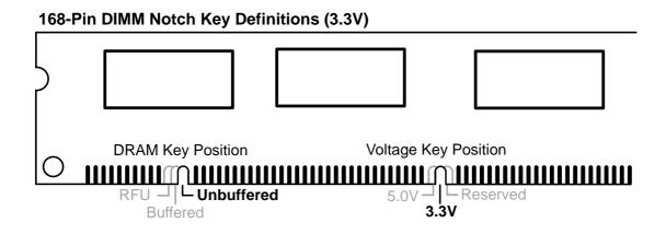
The notches on the DIMM will shift between left, center, or right to identify the type and also to prevent the wrong type from being inserted into the DIMM slot on the motherboard. You must ask your retailer the correct DIMM type before purchasing. This motherboard supports four clock signals per DIMM slot.
