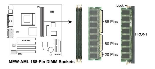
The DIMMs must be **3.3V Unbuffered** for this motherboard. To determine the DIMM type, check the notches on the DIMMs (see figure below).
