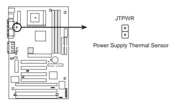
**MEB Thermal Sensor Connector**
