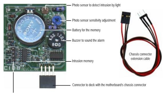
Two switch connectors to detect intrusion by chassis mounted micro switches
