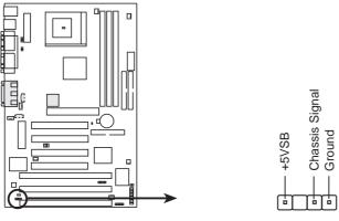
**MEB Chassis Open Alarm Lead**
