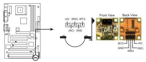
**MEB Infrared Module Connector**
