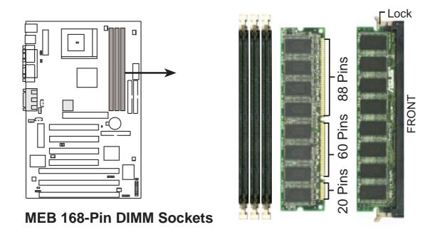
The DIMMs must be **3.3V Unbuffered** for this motherboard. To determine the DIMM type, check the notches on the DIMMs (see figure below).
