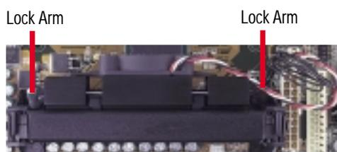
**WARNING!** Make sure the heatsink is mounted tightly against the SECC2, SECC, or SEPP; otherwise, the CPU will overheat. You may install an auxiliary fan to provide adequate circulation across the processor's passive heatsink.
