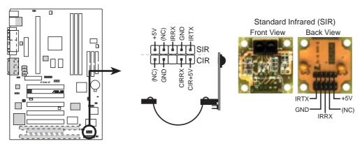
**P3W-E Infrared Module Connector**
