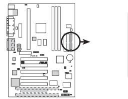
**NOTE:** Orient the red markings on the floppy ribbon cable to PIN 1
