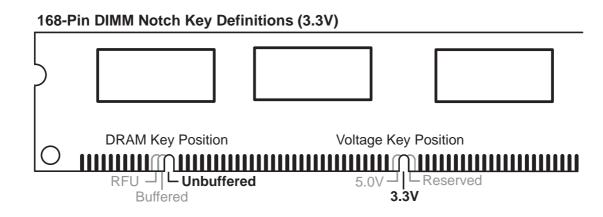
The notches on the DIMM module will shift between left, center, or right to identify the type and also to prevent the wrong type from being inserted into the DIMM slot on the motherboard. You must ask your retailer the correct DIMM type before purchasing. This motherboard supports four clock signals per DIMM slot.
