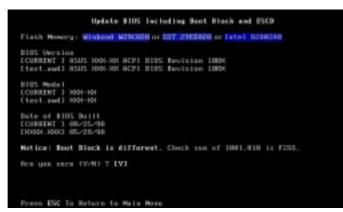
7. The utility starts to program the new BIOS information into the flash ROM. The boot block will be updated automatically only when necessary. This will minimize the chance that a failed update will prevent your system from booting up. When the programming is finished, *Flashed Successfully* will be displayed.
