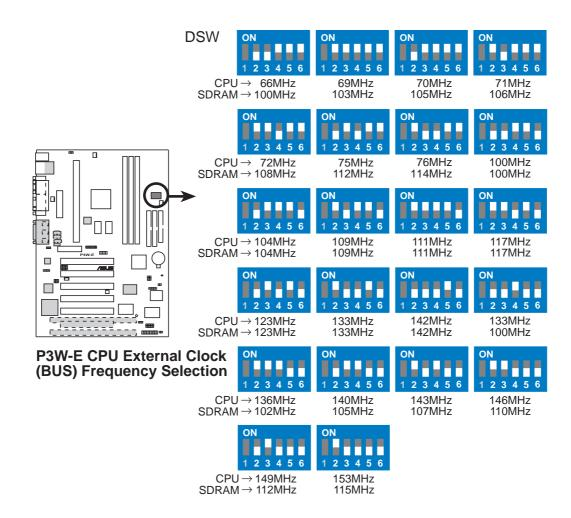
**WARNING!** CPU frequencies other than 66MHz, 100MHz, and 133MHz are not guaranteed to be stable. Premature wearing of the processor may result when overclocking. Be sure that the DIMM you use can handle the specified SDRAM MHz or else bootup will not be possible.
