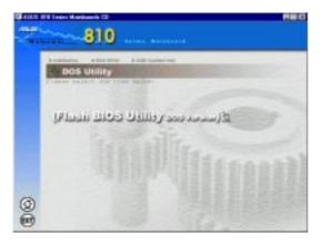
**Flash BIOS Utility (DOS Version):** Provides information on the Flash BIOS utility (AFLASH.EXE). Choose "Restart in MS-DOS mode" then type "aflash" from the AFLASH folder on the support CD.
