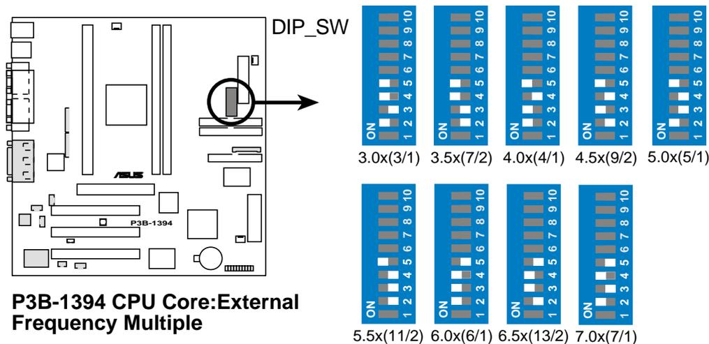
**P3B-1394 CPU Core:External Frequency Multiple**
