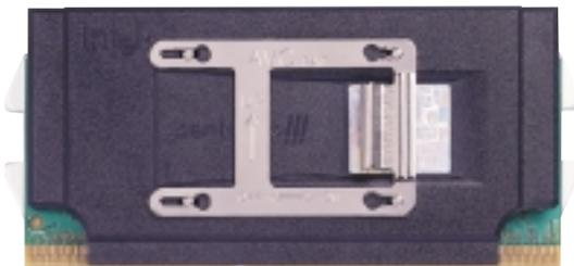
Example of an incorrectly installed retention clip
