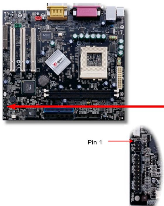
Attach the power LED, EMPI, speaker, power and reset switch connectors to the corresponding pins. If you enable "[Suspend Mode](#)" item in BIOS Setup, the ACPI & Power LED will keep flashing while the system is in suspend mode.
