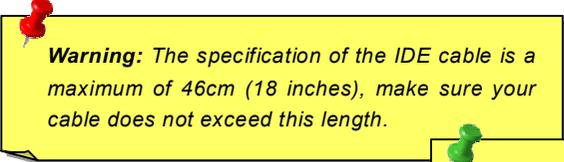
**Warning:** The specification of the IDE cable is a maximum of 46cm (18 inches), make sure your cable does not exceed this length.
