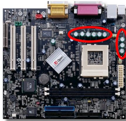
The power circuit of the CPU core voltage must be checked to ensure system stability for high speed CPUs (such as the new Pentium III, or when overclocking). A typical CPU core voltage is 2.0V, so a good design should control voltage between 1.860V and 2.140V. That is, the transient must be below 280mV. Below is a timing diagram captured by a Digital Storage Scope, it shows the voltage transient is only 143mV even when maximum 18A current is applied.
