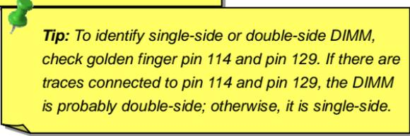
**Tip:** To identify single-side or double-side DIMM, check golden finger pin 114 and pin 129. If there are traces connected to pin 114 and pin 129, the DIMM is probably double-side; otherwise, it is single-side.
