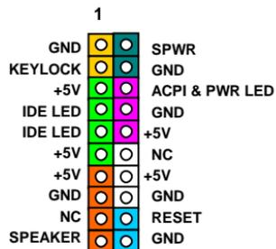
Attach the power LED, keylock, speaker, and reset switch connectors to the corresponding pins. If you enable Power Management > [Suspend Mode](#) in BIOS Setup, the ACPI & Power LED will keep flashing while the system is in suspend mode.
