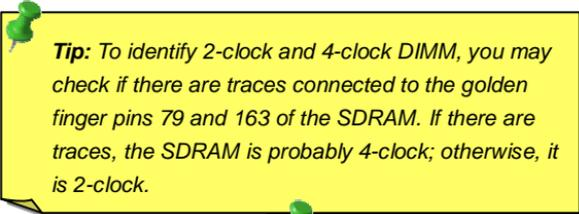
**Tip:** To identify 2-clock and 4-clock DIMM, you may check if there are traces connected to the golden finger pins 79 and 163 of the SDRAM. If there are traces, the SDRAM is probably 4-clock; otherwise, it is 2-clock.
