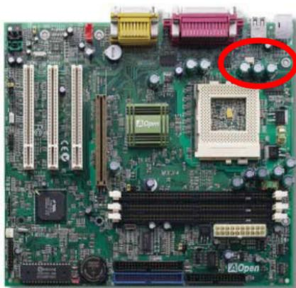
The power circuit of the CPU core voltage must be checked to ensure system stability for high speed CPUs (such as the new Pentium III, or when overclocking). A typical CPU core voltage is 2.0V, so a good design should control voltage between 1.860V and 2.140V. That is, the transient must be below 280mV. Below is a timing diagram captured by a Digital Storage Scope, it shows the voltage transient is only 143mV even when maximum 18A current is applied.
