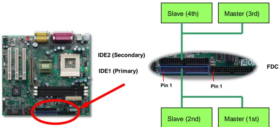
IDE1 is also known as the primary channel and IDE2 as the secondary channel. Each channel supports two IDE devices that make a total of four devices. In order to work together, the two devices on each channel must be set differently to **master** and **slave** mode. Either one can be the hard disk or the CDROM. The setting as master or slave mode depends on the jumper on your IDE device, so please refer to your hard disk and CDROM manual accordingly.
