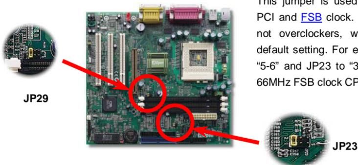
This jumper is used to specify the relationship of PCI and [FSB](#) clock. Generally speaking, if you are not overclockers, we recommend to set at the default setting. For example, you must set JP29 to "5-6" and JP23 to "3-4" if you want to overclock a 66MHz FSB clock CPU to 100MHz or higher.
