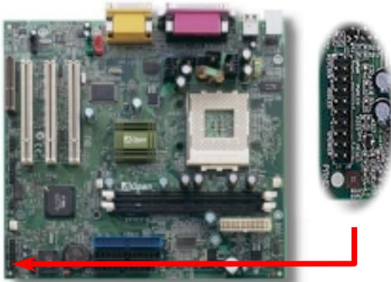
Attach power LED, EMPI, speaker, power and reset switch connectors to the corresponding pins. If you enable "[Suspend Mode](#)" item in BIOS Setup, the ACPI & Power LED will keep flashing while the system is in suspend mode.
