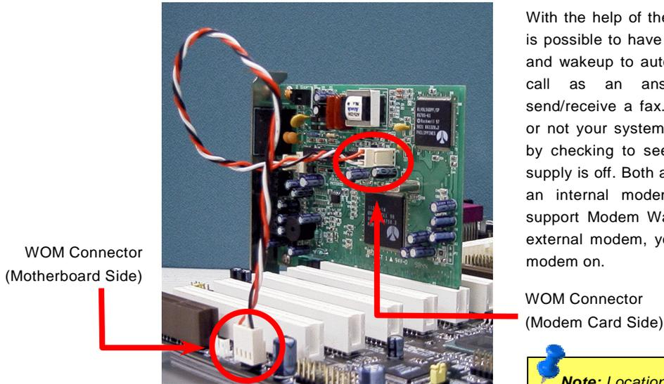
With the help of the ATX soft power On/Off, it is possible to have a system totally power off, and wakeup to automatically answer a phone call as an answering machine or to send/receive a fax. You may identify whether or not your system is in true power off mode by checking to see if the fan of your power supply is off. Both an external box modem and an internal modem card can be used to support Modem Wake Up, but if you use an external modem, you have to leave your box modem on.
