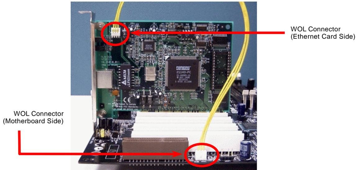
**Note:** Location of WOL connectors on both motherboard and modem card may be different from the illustration due to various motherboards and modem cards.
