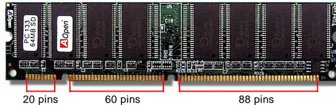
2. Insert the module straight down to the DIMM slot with both hands and press down firmly until the DIMM module is securely in place.
