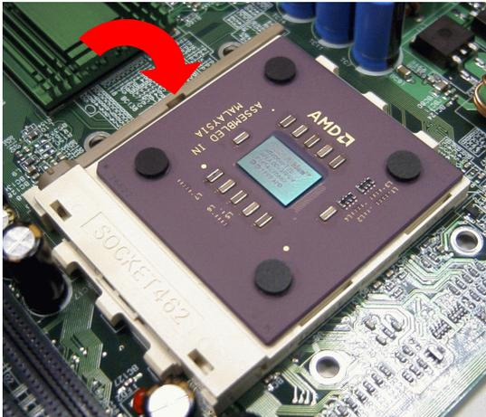
**Note:** If you do not match the CPU socket Pin 1 and CPU cut edge well, it may damage the CPU.
