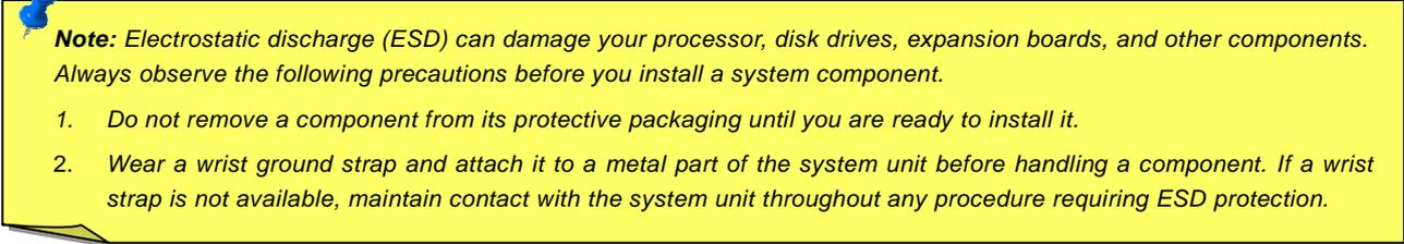
**Note:** *Electrostatic discharge (ESD) can damage your processor, disk drives, expansion boards, and other components. Always observe the following precautions before you install a system component.*
