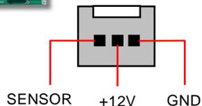
**Note:** Some CPU fans do not have sensor pin, so that cannot support fan monitoring.
