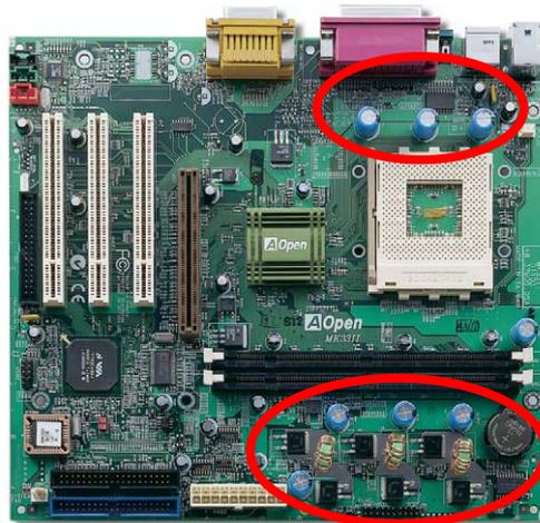
The power circuit of the CPU core voltage must be checked to ensure system stability for high speed CPUs (such as the new Pentium III, or when overclocking). A typical CPU core voltage is 2.0V, so a good design should control voltage between 1.860V and 2.140V. That is, the transient is below 280mV. Below is a timing diagram captured by a Digital Storage Scope, it shows the voltage transient is only 143mV even when maximum 18A current is applied.
