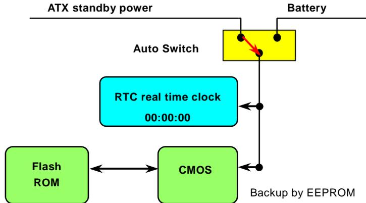
Auto switching to ATX standby power as long as AC power line is plugged. This smart design increases battery life if you still plug battery on motherboard.
