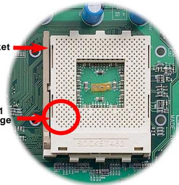
2. Locate Pin 1 in the socket and look for a black dot or cut edge on the CPU upper interface. Match Pin 1 and cut edge, then insert the CPU into the socket.
