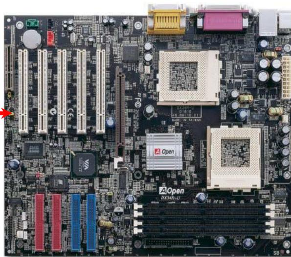
**Note:** Please remove the jumper cap from the Front Panel Audio Connector before you connect the cable. Do not remove this yellow jumper cap if housing without an audio port on the front panel.
