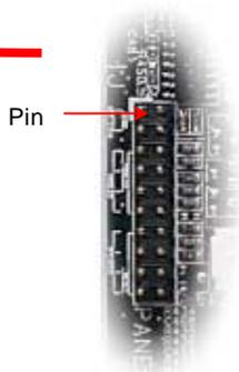
Attach the power LED, speaker, power and reset switch connectors to the corresponding pins. If you enable “Suspend Mode” item in BIOS Setup, the ACPI & Power LED will keep flashing while the system is in suspend mode.
