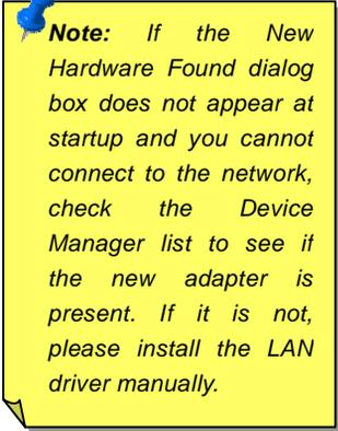
**Note:** *If the New Hardware Found dialog box does not appear at startup and you cannot connect to the network, check the Device Manager list to see if the new adapter is present. If it is not, please install the LAN driver manually.*
