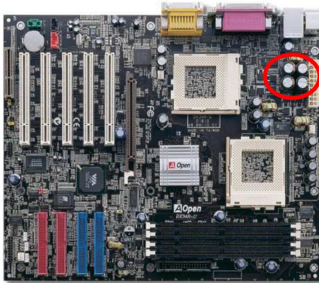
The power circuit of the CPU core voltage must be checked to ensure system stability for high speed CPUs (such as the new Pentium III, or when overclocking). A typical CPU core voltage is 2.0V, so a good design should control voltage between 1.860V and 2.140V. That is, the transient must be below 280mV. Below is a timing diagram captured by a Digital Storage Scope, it shows the voltage transient is only 143mV even when maximum 18A current is applied.
