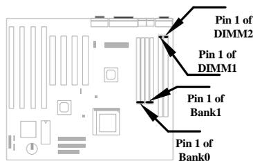
This mainboard has four 72 pin SIMM sockets (Single-in-line Memory Module) and two 168 pin DIMM socket (Dual-in-line Memory Module) that allow you to install system memory from minimum 8MB up to maximum 256MB.
