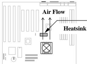
Attach the heatsink and fan to the CPU. Check its orientation, make sure the air flow go through the heatsink.
