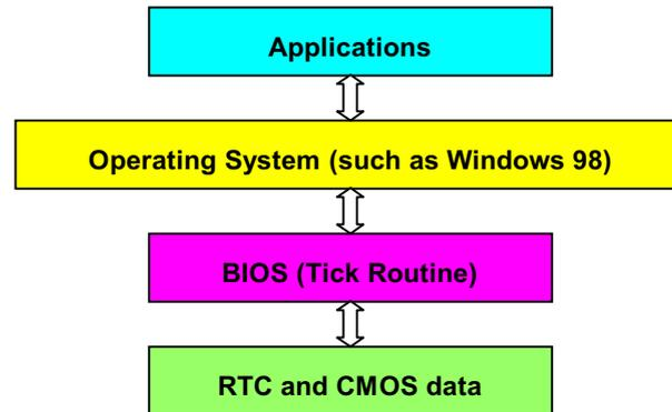
There is a Tick Routine (that goes live around every 50m sec) in the BIOS to keep record of date/time information. In general the BIOS, this Tick Routine does not update the CMOS every time because the CMOS is a very slow device that degrades system performance. The Tick Routine of the AOpen BIOS has 4 digits for year coding, as long as applications and the operating system
