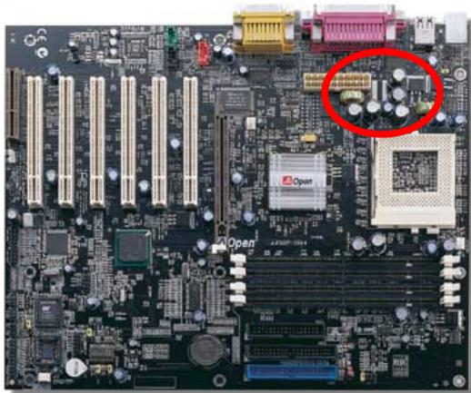
The power circuit of the CPU core voltage must be checked to ensure system stability for high speed CPUs (such as the new Pentium III, or when overclocking). A typical CPU core voltage is 2.0V, so a good design should control voltage between 1.860V and 2.140V. That is, the transient is below 280mV. Below is a timing diagram captured by a Digital Storage Scope, it shows the voltage transient is only 143mV even when maximum 18A current is applied.
