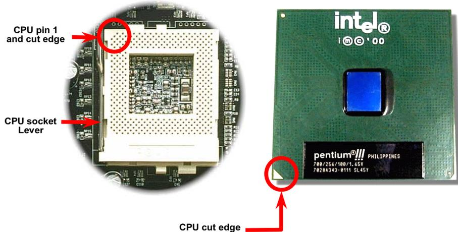
3. Press down the CPU socket level and finish CPU installation.
