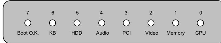
The total 8 LEDs light up alternatively if the system fails in one of eight stages. Once the LED7 (latest LED) is lit, this indicates that the system has completed its boot-up procedure.
