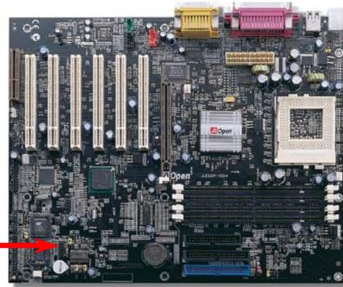
**Note:** Please remove the jumper cap from the Front Panel Audio Connector before you connect the cable. Do not remove this yellow jumper cap if housing without an audio port on the front panel.
