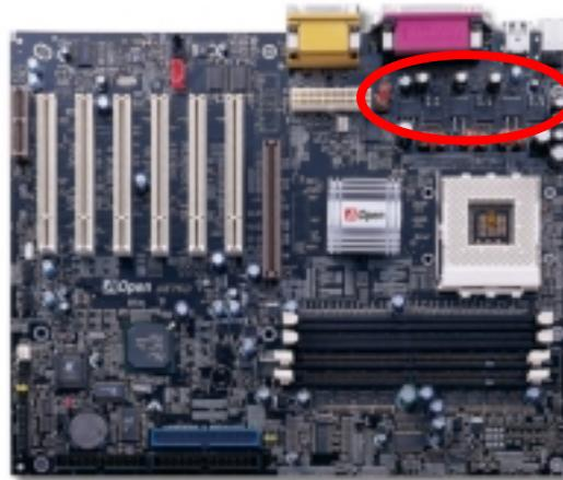
The power circuit of the CPU core voltage must be checked to ensure system stability for high speed CPUs (such as the new Pentium 4, or when overclocking). A typical CPU core voltage is 2.0V, so a good design should control voltage between 1.860V and 2.140V. That is, the transient must be below 280mV. Below is a timing diagram captured by a Digital Storage Scope which shows the voltage transient is only 143mV even when maximum 18A current is applied.
