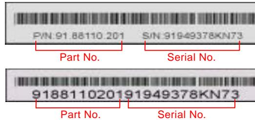
**P/N: 91.88110.201** is part number, **S/N: 91949378KN73** is serial number.
