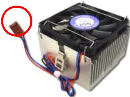
**Note:** You must using 3-pin CPU cooler fan with this motherboard. Only 3-pin cooler fan has support hardware monitoring function.
