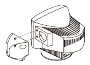
Unlike ordinary speakers, the speakers that came with your Aspire system do not use a power adapter. Instead, it shares power with your system via the USB interface.
