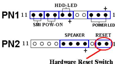
Attach the cable from the case's front panel Reset switch to this header. Press and hold the reset button for at least one second to reset the system.
