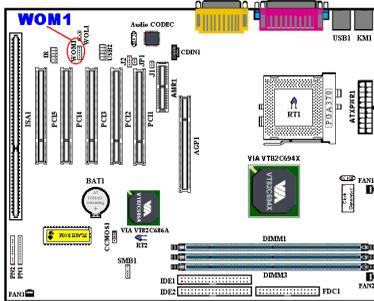
If you have an internal modem adapter that supports this feature, then you can connect the specific cable from the internal modem adapter to this header. This feature lets you wake up your computer via remote control through the modem.
