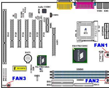
Attach the connector from the individual CPU fan to the header named FAN1, connector from the chassis fan to the header FAN3 and attach the connector from the power fan to FAN2 header.
