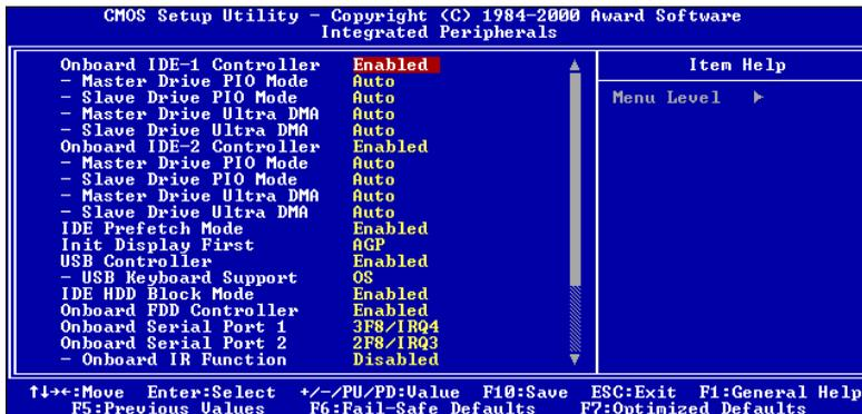
Figure 3-6A. Integrated Peripherals Menu Upper Screen
