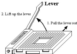
Figure 2-3. Socket 370 and open its lever
