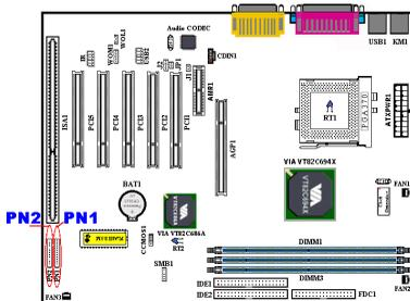
PN1 and PN2 are for switches and indicators for the chassis’s front panel, there are several functions that come from these two headers. You have to watch the pin position and the orientation, or you may cause system malfunctions. Figure 2-9 shows you the PN1 and PN2 functions of the pins.
