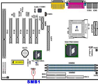
This connector is reserved for system management bus (SM bus). The SM bus is a specific implementation of an I<sup>2</sup>C bus. I<sup>2</sup>C is a multi-master bus, which means that multiple chips can be connected to the same bus and each one can act as a master by initiating a data transfer. If more than one master simultaneously tries to control the bus, an arbitration procedure decides which master gets priority.
