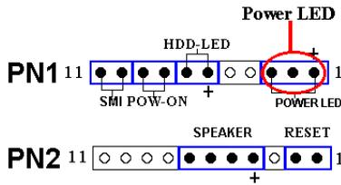
There is a specific orientation for pins 1 through 3. Insert the three-threaded power LED cable to pins 1~3. Check to make sure the correct pins go to the correct connectors on the motherboard. If you install them in the wrong direction, the power LED light will not illuminate correctly.
