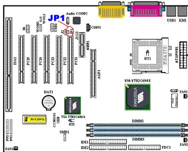
This header can select whether the AMR card insertion on the AMR slot is primary or secondary. When you don’t want to use the onboard audio CODEC, you have to set JP1 at open. The default setting is short. Remember that only when using an MC 97 card should you select the JP1 as open. Otherwise, leave it selected as short.
