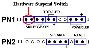
Attach the cable from the case's front panel suspend switch (if there is one) to this header. Use this switch to enable/disable the power management function by hardware.
