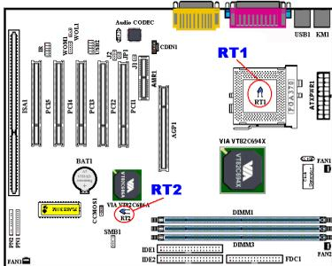
The RT1 thermistor used to detect the CPU temperature.
