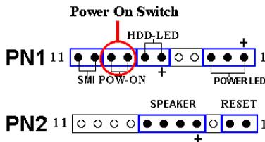
Attach the cable from the case's front panel power switch to this header.
