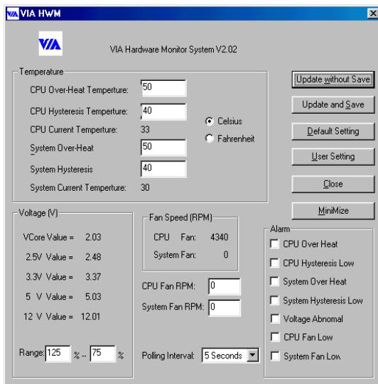
This screen shows the VIA hardware monitor system screen. It shows the information about system temperature, voltages and fan speed. Some items can let you set the warning range; you can accordance your system to make optimize value setting.
