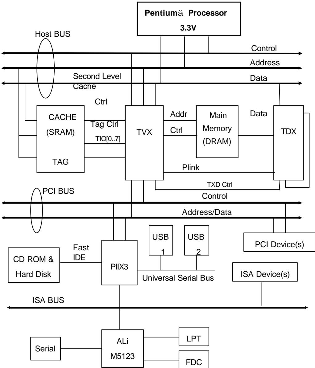
Fig. 1-3 System block diagram
