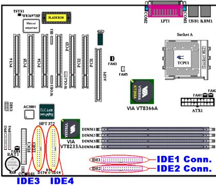
allows for four additional IDE devices in your computer system. Especially, if you want to connect two or four HDDs to get RAID functions, it is very convenient for you to install the HDDs to IDE3 and IDE4. See the Chapter 4 for detailed information about RAID settings.
