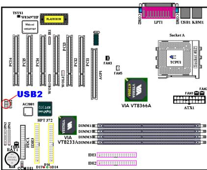
This header is for connecting the additional USB port plugs. You can use the special USB port expansion cable. It provides four additional USB plugs. These USB plugs can be fixed on the back panel.
