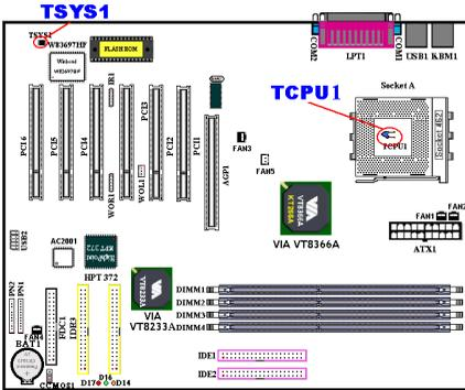
The TCPUI is used to detect the CPU temperature. The TSYS1 is used to detect the system environment temperature. You can see the readings in the BIOS or in the hardware monitoring application main screen.
