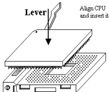
**Figure 2-2. Install the CPU into socket A**
