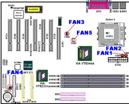
Attach the connector from the CPU fan to the header named FAN1 and connector from the chassis fan to the header FAN2 (These two fan headers have a sense signal that can detect fan rotation speeds) or FAN4 and attach the connector from the power fan to FAN3 header. FAN5 is for the northbridge chipset fan.
