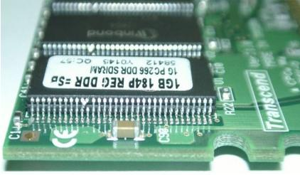
Most of the DDR memory 1GB modules available now consist of 64 M x 4 chip, which can't be used on KR7A-133/KR7A-133R motherboard. Before purchasing the memory module, we suggest users carefully check out the memory specification, which should be provided by memory module vendor. The left picture illustrates a DDR 1 GB module made by 64 M x 4 chip and special technology- stacking two memory chips together. This kind of memory can't be supported by VIA KT266A chipset.
