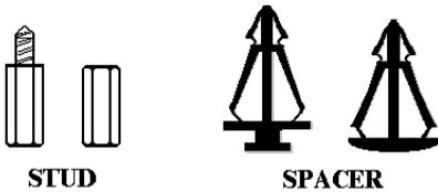
**Figure 2-3. The outline of stud and spacer**
