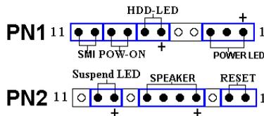
Figure 2-9. The definition of PN1 and PN2 pins
