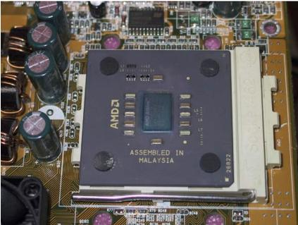
First, install the processor into the processor socket.
