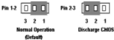
Figure 2-8. CCMOS1 jumper setting
