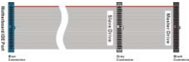
Figure 2-10. Ultra DMA 66 Ribbon Cable Outline
