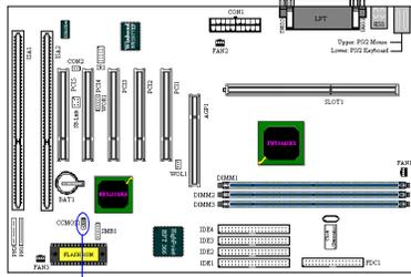
Jumper CCMOS1 discharge CMOS memory. When you install the motherboard, make sure this jumper is set for normal operation (pin 1 and 2 shorted). See figure 2-6.
