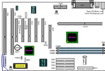
PN1 and PN2 are for switches and indicators for the chassis's front panel, there are several functions that come from these two headers. You have to watch the pin position and the orientation, or you may cause system malfunctions. Figure 2-7 shows you the PN1 and PN2 functions of the pins.
