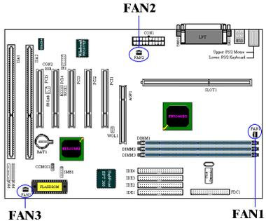
Attach the connector from the individual CPU fan to the header named FAN2, and attach the connector from the chassis fan to FAN1 or & FAN3 header.
