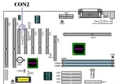
This header is for you to connect an additional thermistor to detect the CPU temperature. You can attach one end of the two-threaded thermal cable that comes with the motherboard to CON2 header, then tape the other end of thermal cable on CPU's heat sink.
