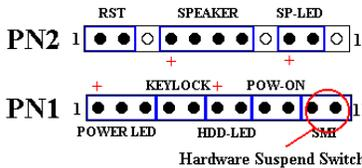
Attach the cable from the case's front panel suspend switch (if there is one) to this header. Use this switch to enable/disable the power management function by hardware.
