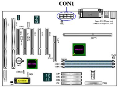
Attach the connector from the power supply to the CON1 connector here. Remember you have to push the connector from the ATX power supply firmly to the end with the CON1 connector, insuring that you have a good connection.
