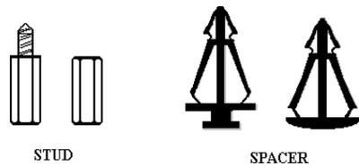
Figure 2-1. The outline of stub and spacer
