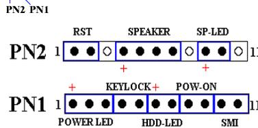
**Figure 2-7. The definition of PN1 and PN2 pins**
