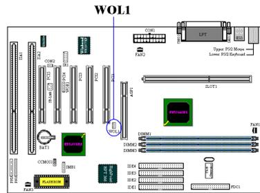
If you have a Network adapter that supports this feature, then you can connect the specific cable from the network adapter to this header. This feature lets you wake up your computer via remote control through a local area network. You may need a specific utility to control the wake up event, like using the Intel® LDCM® utility or other similar utilities.
