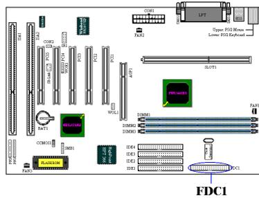
This 34-pin connector is called the “*floppy disk drive connector*”. You can connect a 360K, 5.25”, 1.2M, 5.25”, 720K, 3.5”, 1.44M, 3.5” or 2.88M, 3.5” floppy disk drive, you can even connect a 3 Mode floppy disk drive (it’s a 3 1/2” drive used in Japanese computer systems).
