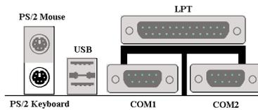
Attach a PS/2 keyboard connector to this 6-pin Din-connector. If you use an AT keyboard, you can go to a computer store to purchase an AT to ATX converter adapter, then you can connect your AT keyboard to this connector. We suggest you use a PS/2 keyboard for best compatibility.
