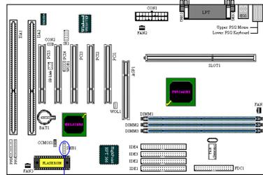
This connector is reserved for system management bus (SMBus). The SMBus is a specific implementation of an I<sup>2</sup>C bus. I<sup>2</sup>C is a multi-master bus, which means that multiple chips can be connected to the same bus and each one can act as a master by initiating a data transfer. If more than one master simultaneously tries to control the bus, an arbitration procedure decides which
