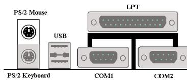
Attach a PS/2 mouse to this 6-pin Din-connector.
