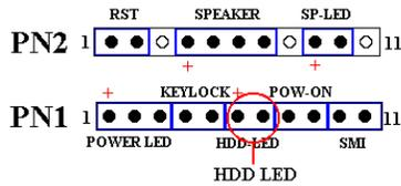
Attach the cable from the case's front panel HDD LED to this header. If you install it in the wrong direction, the LED light will not illuminate correctly.
