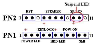
Insert the two-threaded suspend LED cable into pin 9 and pin 10. If you install it in the wrong direction, the LED light will not illuminate correctly.
