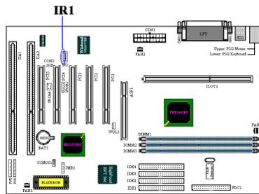
There is a specific orientation for pins 1 through 5, attach the connector from the IR KIT or IR device to the IR1 header (left row only) This motherboard supports standard IR transfer rates.
