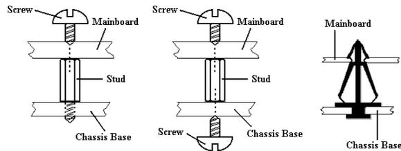
Figure 2-2. The way we fixed the motherboard
