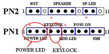
There is a specific orientation for pins 1 through 3. Insert the three-threaded power LED cable to pins 1~3, and the two-threaded keylock cable into pin 4 and pin 5. Check to make sure the correct pins go to the correct connectors on the motherboard. If you install them with the wrong direction, the power LED light will not illuminate correctly.
