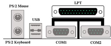
This parallel port is also called an “LPT” port, because it usually connects to the printer. You can connect other devices that support this communication protocol, like a scanner, M.O. drive, etc.
