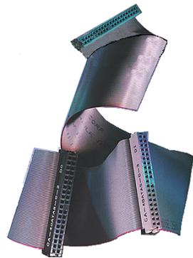
**Figure 2-9. Photo of an Ultra ATA/66 Conductor Cable**
