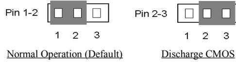
**Figure 2-6. CCMOS1 jumper setting**
