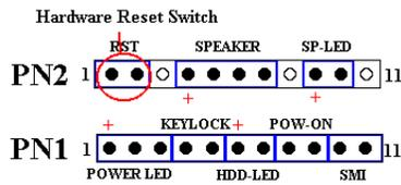
Attach the cable from the case's front panel Reset switch to this header. Press and hold the reset button for at least one second to reset the system.
