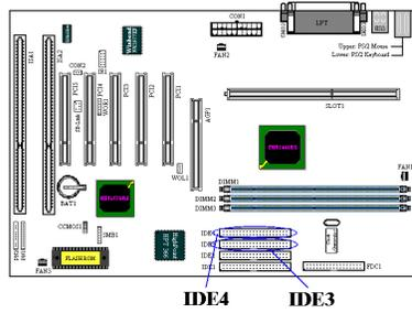
The BE6 supports the Ultra ATA/66 (Also known as Ultra DMA/66) specification. It enhances existing Ultra ATA/33 technology by increasing both performance and data integrity. This new high-speed interface doubles the Ultra ATA/33 burst data transfer rate to 66.6 Mbytes/sec. The result is maximum disc performance using the current PCI local bus environment. Figure 2-8 shows you the different between the Ultra ATA/33 and Ultra ATA/66 Conductor Cable.
