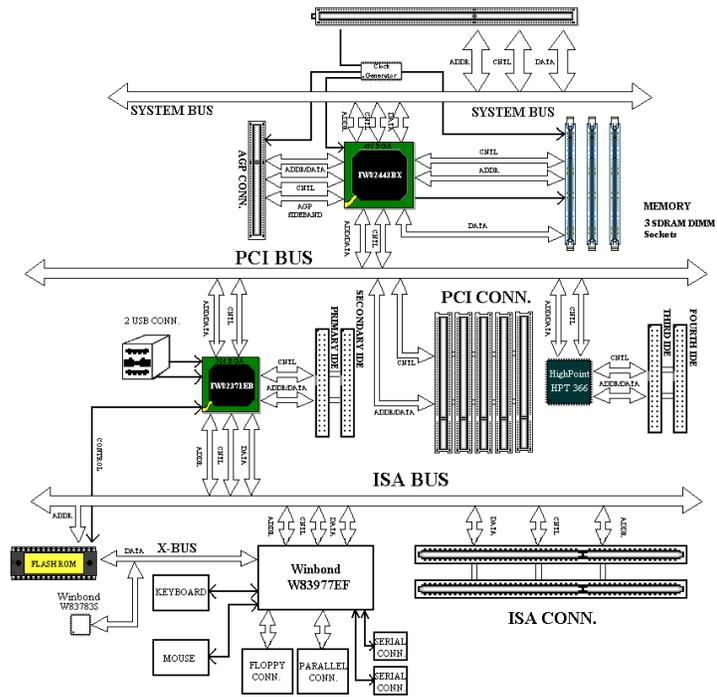
Figure 1-3. System diagram of the 440BX chipset
