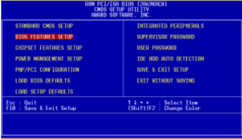
By choosing the BIOS FEATURES SETUP option from the INITIAL SETUP SCREEN menu, the screen below is displayed.
