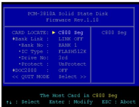
If you install more than one PCM-3810A in your system, and each PCM-3810A has its own memory address, the "card locate" function allows you to modify each PCM-3810A as follows:
