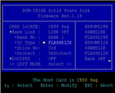
The "IC Type" option allows you to set the type of ICs which you are going to install or have installed on the bank you are modifying. If you want to install a DOC 2000 on the PCM-3810A, refer to the "DOC 2000" option.
