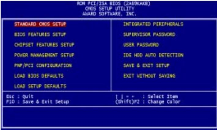
When you choose the STANDARD CMOS SETUP option from the INITIAL SETUP SCREEN menu, the screen below is displayed.
