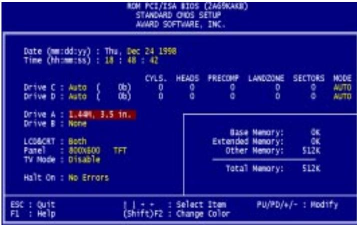
This standard setup menu allows users to configure system components such as the date, time, hard disk drive, floppy drive, display, and memory. Online help for each field can be accessed by pressing F1.
