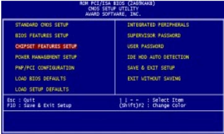
By choosing the CHIPSET FEATURES SETUP option from the INITIAL SETUP SCREEN menu, the screen below is displayed.
