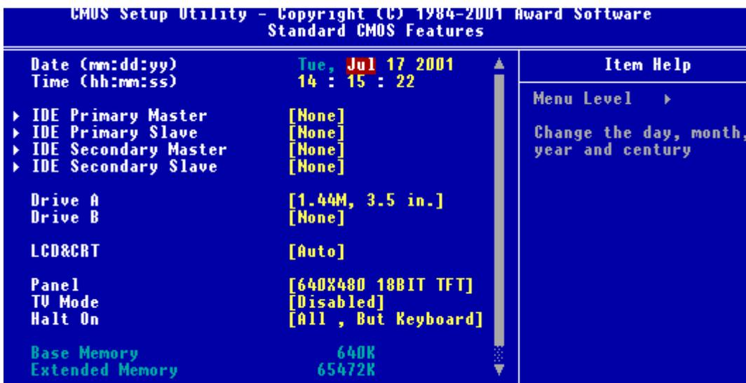
This standard setup menu allows users to configure system components such as the date, time, hard disk drive, floppy drive, display, and memory. Online help for each field can be accessed by pressing F1.
