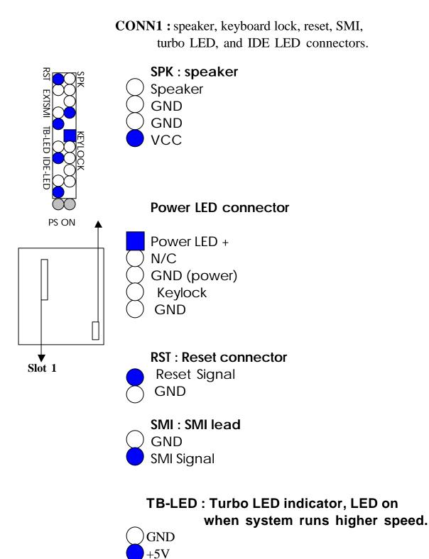
IDE-LED : IDE devices indicator LED connector. IDE-LED stays ON indicates
