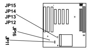
JP11, JP12, JP13, JP14, JP15, JP16 - Power Selection for the CPU Core Voltage, Bus Section and Bus Voltage
