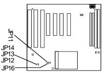
JP11, J12, J13, J14, JP16 - Power Selection for the CPU Core Voltage, Bus Section and Bus Voltage
