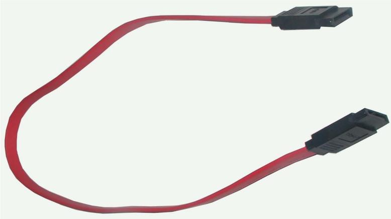
Connect one port of the SATA cable to the mainboard, and connect another port to the SATA Hard Disk.
