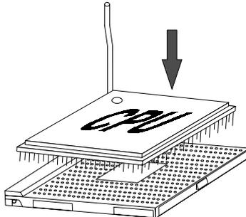
2. If the CPU is correctly installed, the pins should be completely embedded into the socket and can not be seen. Please note that any violation of the correct installation procedures may cause permanent damages to your mainboard.
