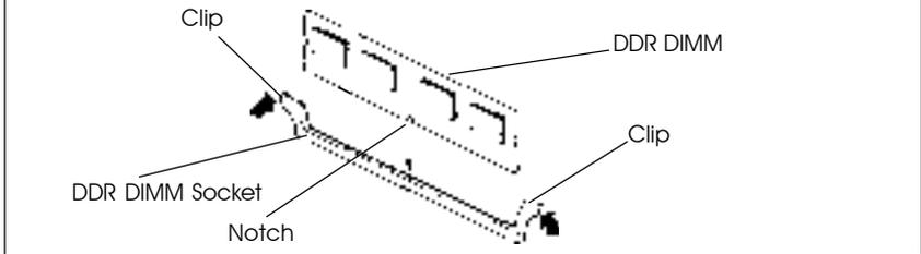
4. Position the DDR DIMM above the socket. Align the notch in the bottom edge of the DDR DIMM with the keys in the socket.
