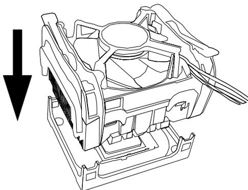
6. Use one end of the clip to hook the latch of the CPU sliding plate and then hook the other three latches to fix the cooling fan set. At last, connect the fan to the power supply connector provided on your mainboard.
