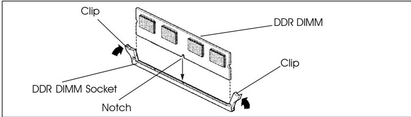
4. Position the DDR DIMM above the socket. Align the notch in the bottom edge of the DDR DIMM with the keys in the socket.
