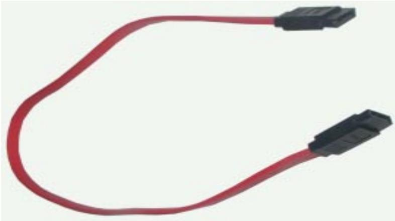
Connect one end of the SATA cable to the mainboard, and connect another end to the SATA Hard Disk.
