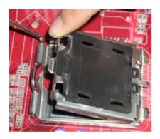
2.Use index finger to lift the top steel shell.
