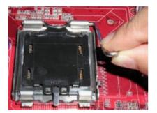
1.Use index finger and thumb to move metal lever so it is separated from the bottom steel shell grip hook.
