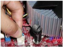
10. At last, attach the fan wire connector to the 4 pin fan header connector on the motherboard labeled CPU FAN.
