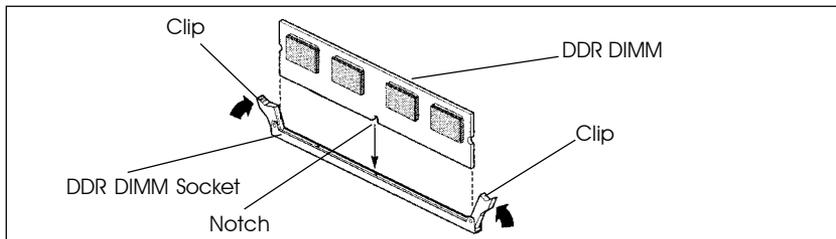
4. Position the DDR DIMM above the socket. Align the two small notches in the bottom edge of the DDR DIMM with the keys in the socket.
