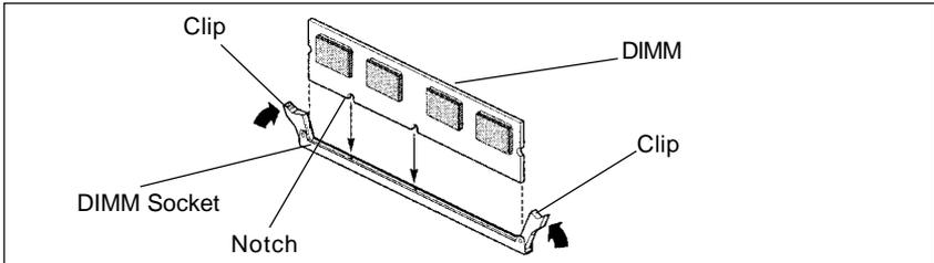
4. Position the DIMM above the socket. Align the two small notches in the bottom edge of the DIMM with the keys in the socket.
