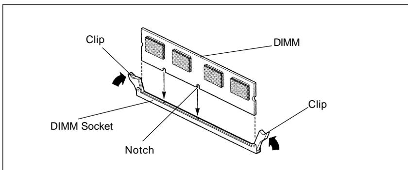
5. Position the DIMM above the socket. Align the two small notches in the bottom edge of the DIMM with the keys in the socket.
