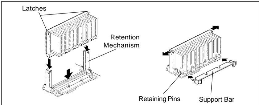
3. Slide the top heatsink support bar onto the retaining pins of the support's base as shown in figure.
