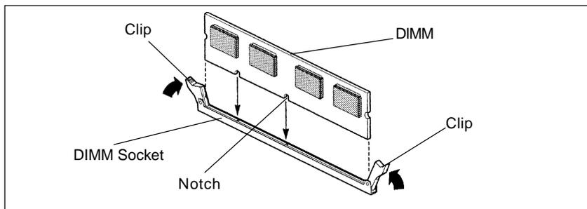
5. Position the DIMM above the socket. Align the two small notches in the bottom edge of the DIMM with the keys in the socket.
