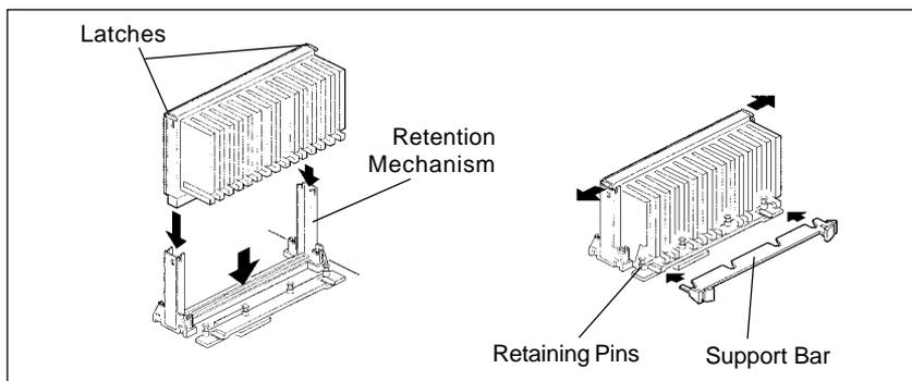
3. Slide the top heatsink support bar onto the retaining pins of the support's base as shown in figure.
