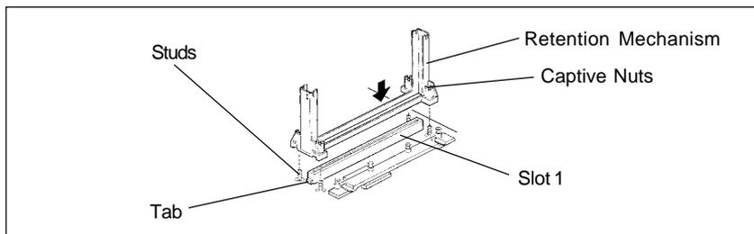
3. Finger tighten all four captive nuts to make sure they start correctly on the threads of the attachment studs.
