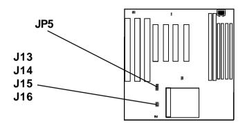
JP5, J13, J14, J15, J16- Power Selection for the CPU Bus Section & CPU Core-Voltage Select
