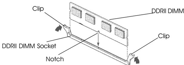
4. Position the DDRII DIMM above the socket. Align the middle notch in the bottom edge of the DDRII DIMM with the key in the socket.
