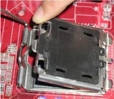
2. Use the index finger to lift the top steel shell.
