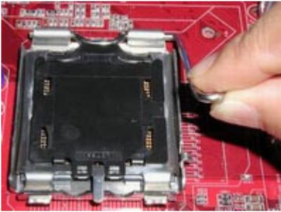
1. Please turn off the power and unplug the power cord before installing the CPU. Use your index finger and thumb, unhook the metal lever from the bottom steel shell grip hook.
