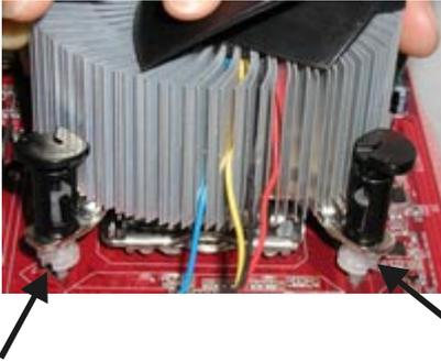
7. Align the fastener tips with the Sapphire motherboard hole pattern, insert the fastener tips into the holes, guiding the wires to avoid pinching. The fasteners will slide through the motherboard holes with no insertion force.
