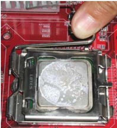
5. Press the metal lever so it is secured in the bottom steel shell grip hook.
