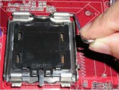
1. Use index finger and thumb to move metal lever so it is separated from the bottom steel shell grip hook.
