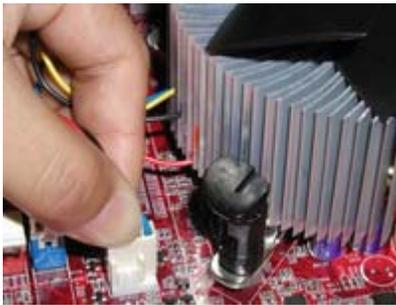
10. At last, attach the fan wire connector to the 4 pin fan header connector on the motherboard labeled CPU FAN.
