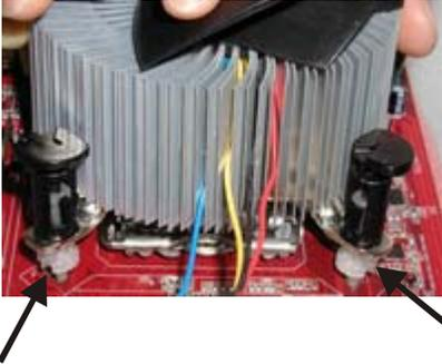
7. Align the fastener tips with the motherboard hole pattern, insert the fastener tips into the holes, guiding the wires to avoid pinching. the fasteners will slide through the motherboard holes with no insertion force.
