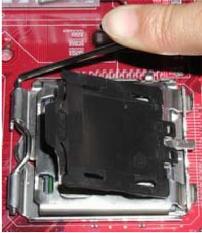
4. Use index finger and thumb to press down metal lever, the cap will be pushed up by the CPU; this may also be done by removing the cap beforehand.
