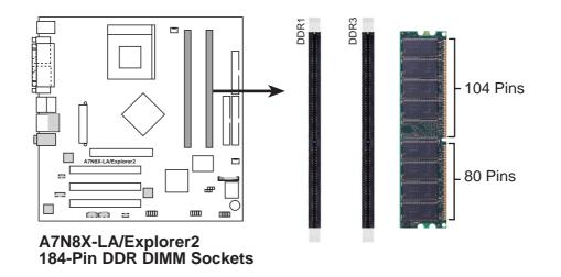
CAUTION: DIMMs are keyed to fit with only one direction. DO NOT force a DIMM into a socket to avoid damaging the DIMM.
