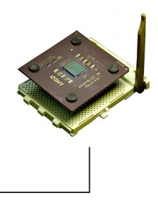
The CPU fits only in one correct orientation. DO NOT force the CPU into the socket to prevent bending the pins and damaging the CPU!
