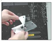
2. Turn over the mainboard, and install the backplate to the proper position.
