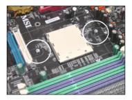
4. Align the retention mechanism and the backplate.
