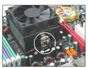
6. Locate the Fix Lever, Safety Hook and the Fixed Bolt.
