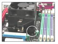
9. Attach the CPU Fan cable to the CPU fan connector on the mainboard.
