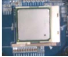
Now with the processor properly installed, you can proceed to install the heatsink. It is important to note that if you have never installed a heatsink on an Intel PIII or Celeron processor before it may be difficult. We recommend you do a dry run a few times before doing the final installation. To allow you to do this read the following instructions. Do not remove the film on the thermally conductive compound until you are ready to do the final installation.
