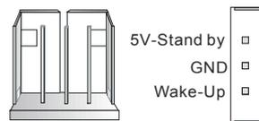
After connecting the WOM cable from your modem to the WOM header, you can set the BIOS to allow the system to wake up when the Modem Card receives a Ring signal.
