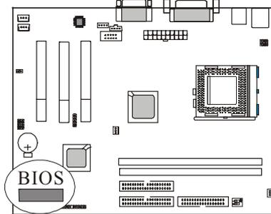
The BIOS IC is inserted in an IC socket, which means that it can be removed and exchanged for another IC if necessary.
