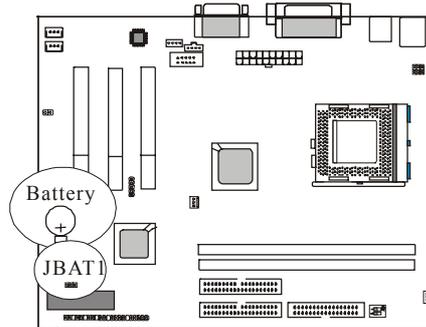
Normally JBAT1 will be in the 1-2 position, this will connect the battery to the southbridge of the chipset which contains the CMOS memory. If JBAT1 is temporarily set to 2-3 this will interrupt the battery electricity flow, and the CMOS memory will be erased, this will however only work if the power supply is not switched on. Now at the next reboot the BIOS will automatically load the CMOS default values.
