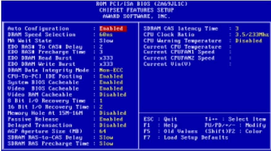
**AUTO CONFIGURATION** [THE BIOS WILL AUTOMATICALLY DETECT THE CPU SPEED AND WILL AUTO-CONFIGURATE THE BUS FREQUENCY, DRAM SPEED, CACHE AND READ/WRITE CYCLE.]
