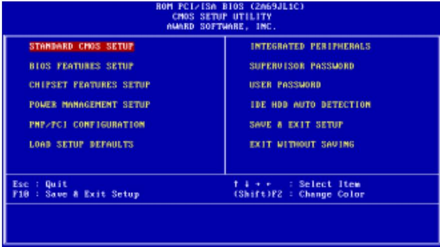
THE MENU DISPLAYS ALL THE MAJOR SELECTION ITEMS AND ALLOW USER TO SELECT ANY ONE OF SHOWN ITEM. THE SELECTION IS MADE BY MOVING CURSOR( PRESS ANY DIRECTION KEY ) TO THE ITEM AND PRESS <ENTER> KEY. AN ON-LINE HELP MESSAGE IS DISPLAYED AT THE BOTTOM OF THE SCREEN AS CURSOR IS MOVING TO VARIOUS ITEMS WHICH PROVIDES USER BETTER UNDERSTANDING OF EACH FUNCTION. WHEN A SELECTION IS MADE, THE MENU OF SELECTED ITEM WILL APPEAR. SO THE USER CAN MODIFY ASSOCIATED CONFIGURATION PARAMETERS.
