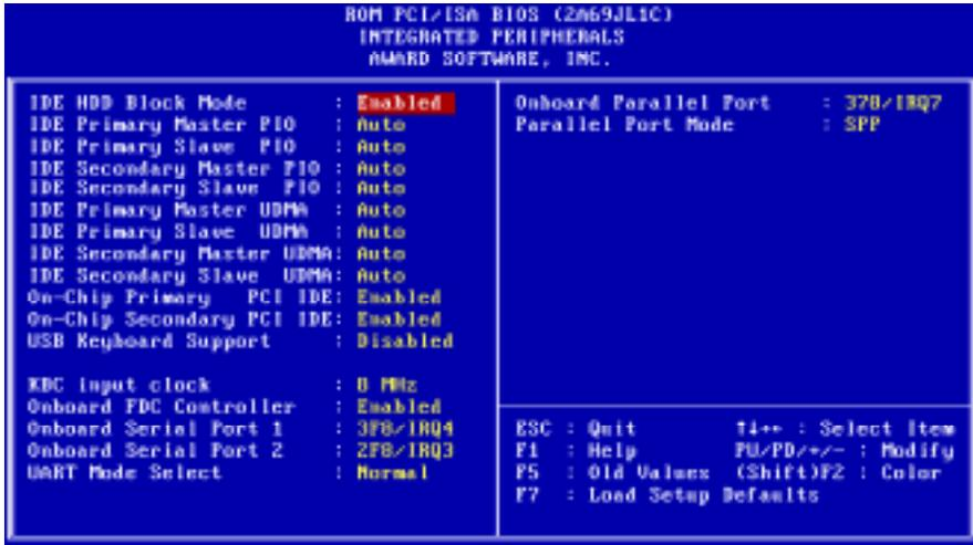
**IDE HDD BLOCK MODE** [THIS FEATURE ENHANCES HARD DISK PERFORMANCE BY MAKING MULTI SECTOR TRANSFER, INSTEAD OF ONE SECTOR PER TRANSFER, MOST OF IDE DRIVERS, EXCEPT VERY EARLY DESIGNS ,CAN USE THIS FEATURE.]
