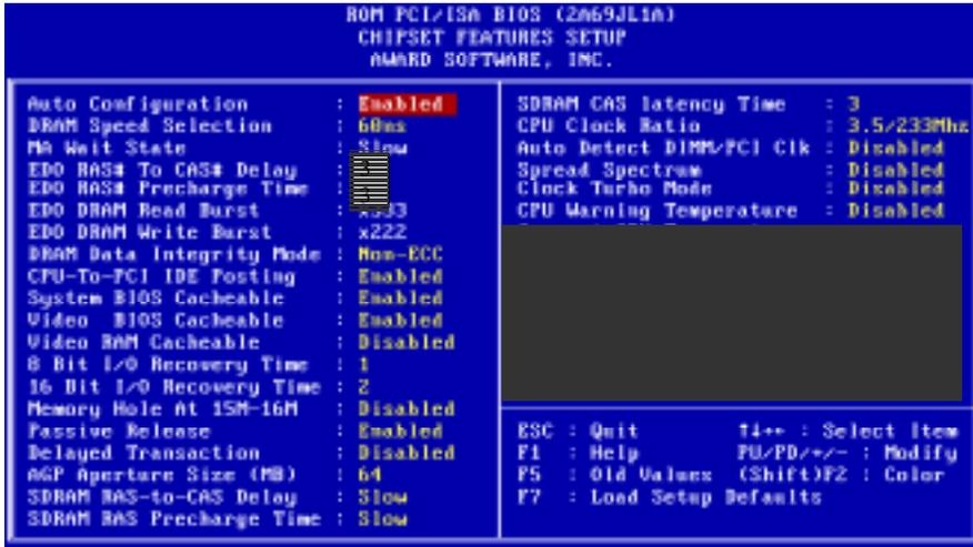
**AUTO CONFIGURATION** [THE BIOS WILL AUTOMATICALLY DETECT THE CPU SPEED AND WILL AUTO-CONFIGURATE THE BUS FREQUENCY, DRAM SPEED, CACHE AND READ/WRITE CYCLE.]
