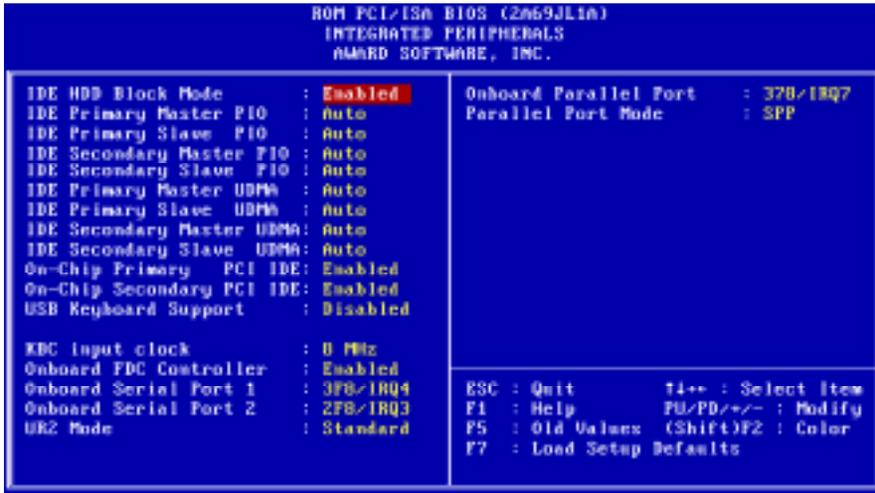
**IDE HDD BLOCK MODE** [THIS FEATURE ENHANCES HARD DISK PERFORMANCE BY MAKING MULTI SECTOR TRANSFER, INSTEAD OF ONE SECTOR PER TRANSFER, MOST OF IDE DRIVERS, EXCEPT VERY EARLY DESIGNS ,CAN USE THIS FEATURE.]
