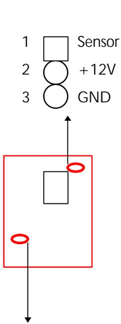
**FAN1 :** CPU cooling fan connector. Wire with +12V voltage (most likely red wire) must be plugged into pin2, and GROUND wires (most likely black wires) must be plugged into pin1 and/or pin3. Please confirm the wire color re-presentation with your supplier.
