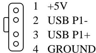
When you'd like to use USB front panel port, please ask your supplier for related accessory. (such as USB front panel connector and front panel USB cable). If it is not available, then you only can use 2 USB ports on the back panel, and set JP10 as default setting ; "1-2, 4-5".
