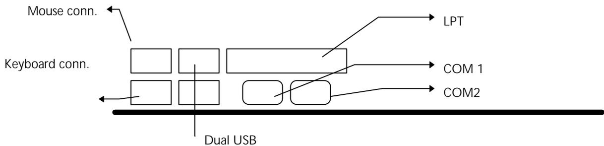
**LPT** : this connector is used to connect parallel port cable.
