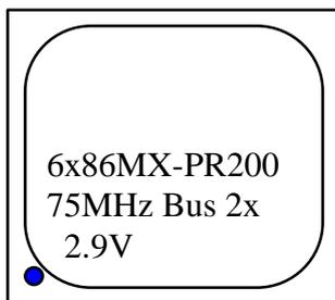
The bottom line of the mark on the processor contains a code 2.9 that identifies the voltage level type. The second line will show the bus MHz and clock multiplier for jumper setting.
