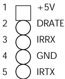
**IR1 :** Infrared module connector.
